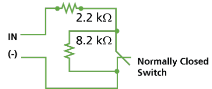
Figure 7: Normally Closed Supervised Input with Double Resistors
